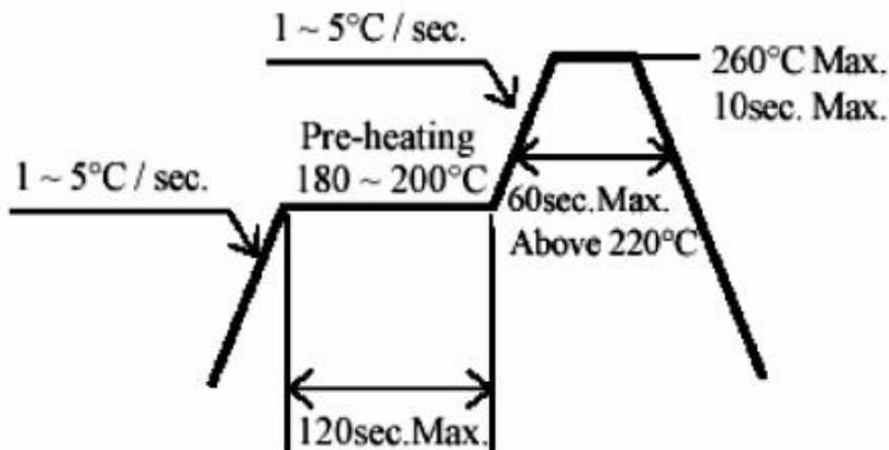
3.2 When soldering, do not put stress on the LEDs during heating. 焊接时，加热期间不要对按压LED.
