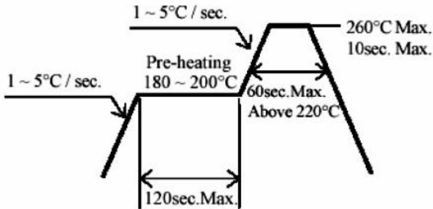
3.2 When soldering, do not put stress on the LEDs during heating. 焊接时，加热期间不要对 LED 施压。
